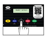
Press the **RED** brew button. Verify the time is correct (4 minutes 36 seconds).
