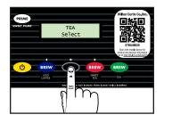
Press the **GREEN** brew button. <u>The time must be set at "1 minute</u> <u>40 seconds</u>". Press the **RED** brew button until the minutes or seconds flashes. Use the **BLACK** button to increase or decrease the time until the time is set to <u>1 minute 40 seconds</u>. Once time is correct press the **RED** brew button until "**ex**" flashes on the display. Then press the **BLACK** button twice, display should read "**Select Brew Button.**" Proceed to step <u>14</u>
