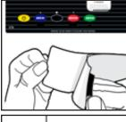
Peel the protective backing off of the new Overlay and attach it to the front of the Brewer Control Panel.
