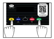
If the display screen is lit on the board, turn **OFF** by pressing the **YELLOW** power button once. To enter the Programming Mode press and hold the **GREEN** brew button. While pressing the **GREEN** brew button, press and hold the **YELLOW** power button for approximately 5 seconds until "**Enter Code**" appears on the display.
